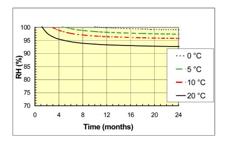
**Fig. 2** Relative humidity of the ambient air (RH) and temperature isopleths as a function of time for start of decay development (mass loss less than 3%) in untreated pine sapwood (Viitanen 1997b).
