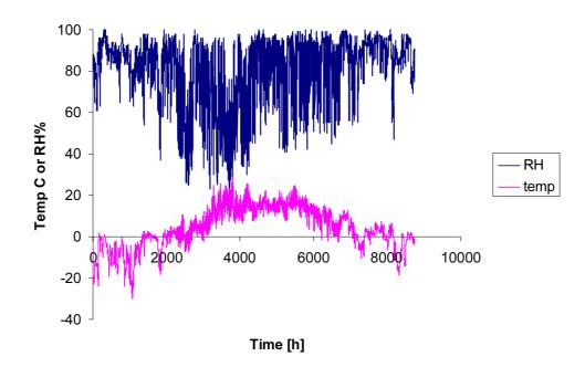
Fig. 6 Measured one-year climate in Helsinki used in the decay modelling example.
