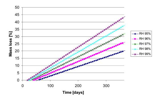
**Fig. 4** Growth of decay as expressed by mass loss at a constant temperature of 15 °C for small untreated pine sapwood samples at different ambient air humidity conditions.
