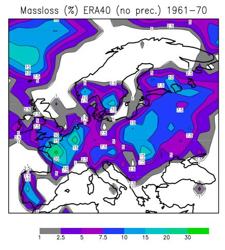
**Fig. 8** Modelled evaluation of mass loss (in %) of pine sapwood that is protected from rain in ten years in Europe.
