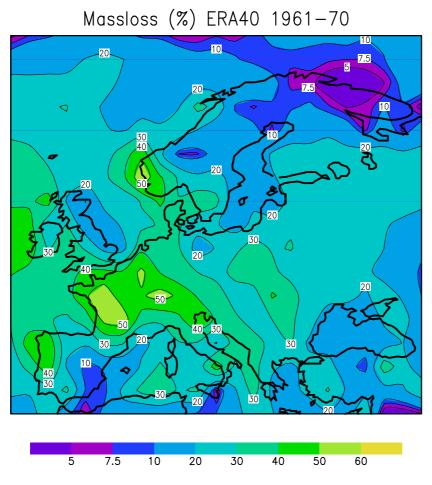
**Fig. 9** Modelled evaluation of mass loss (in %) of pine sapwood that is exposed to rain in ten years in Europe.
