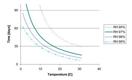
**Fig. 5** Calculated critical time before decay (mass loss process) initiates at different constant temperatures (x-axis) and relative humidity levels of ambient air (different curves).
