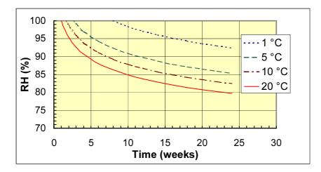
**Fig. 1** Relative humidity of the ambient air (RH) and temperature isopleths as a function of time for start of mould growth in untreated pine sapwood (Viitanen 1997a).
