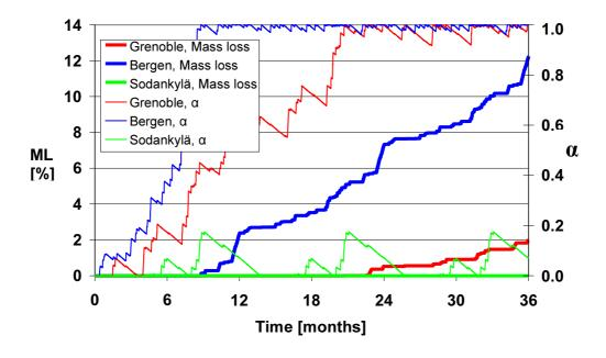
**Fig. 12** Decay development during three years in untreated pine sapwood of a 20 mm thick exterior wooden sheathing at three locations in Europe as modelled using local weather data.
