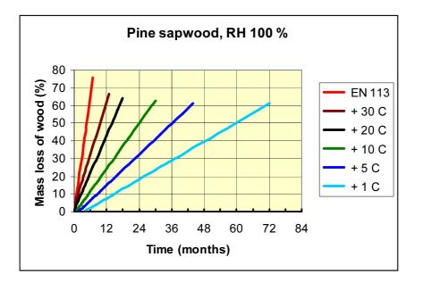
**Fig. 3** Development of decay of *Coniophora puteana* in accelerated decay test (EN 113:1997) and at high humidity (RH 100%) of ambient air at different temperatures. Development of decay is evaluated using mass loss value caused by the fungus in untreated pine sapwood. The curves are fits to the mean values of laboratory test data (Viitanen 1996).
