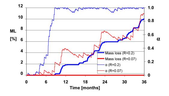
**Fig. 13** Effect of the driving rain exposure coefficient R on the decay development in untreated pine sapwood of a 20 mm exterior wooden sheathing. Weather data for the three years are from Helsinki.
