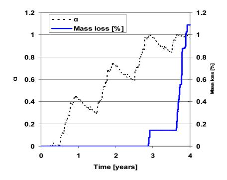
**Fig. 7** Modelled activation and decay in four years based on repeated use of the meteorological data in Fig. 6.
