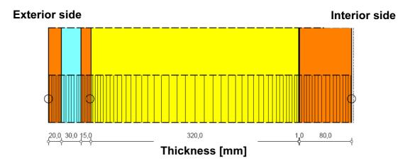
Fig. 11 Cross section of a well-insulated (320 mm) cavity wall with ventilated air cap (30 mm).
