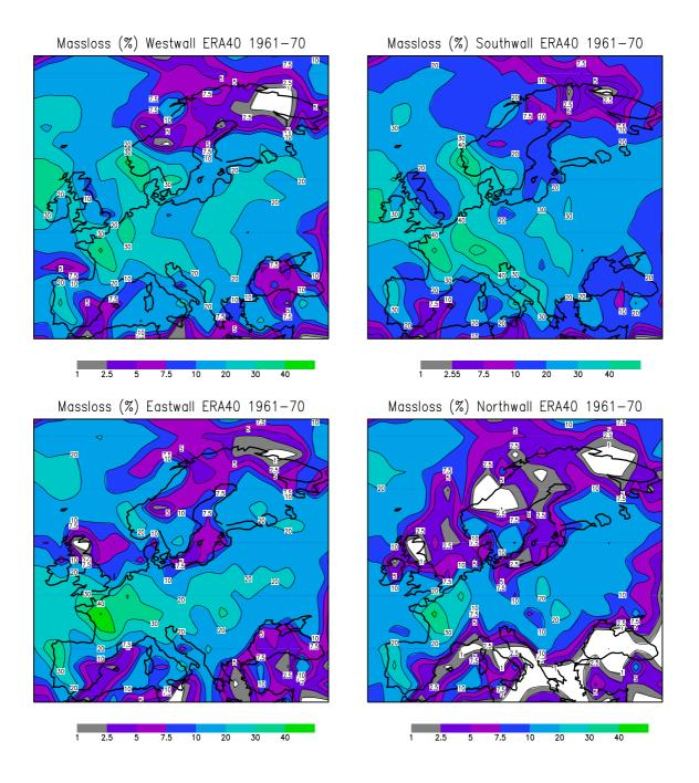
**Fig. 10** Modelled evaluation of mass loss (in %) of pine wood on differently aligned vertical surfaces exposed to driving rain in ten years in Europe.
