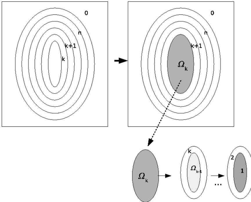
Figure 2. Multi-coated inclusion problem with eigenstrains considering  $n$  phases. Approximation using the average strain fields over  $\Omega_k = V_1 \cup \dots \cup V_k$ , the volume of the composite formed by the phases 1 to  $k$ .
