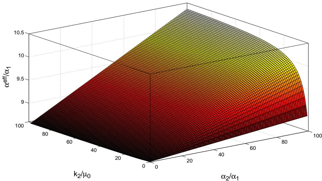
Figure 8. Normalized effective thermal expansion coefficient  $\alpha_{eff}/\alpha_1$  of a composite material made of coated inclusions as described in Fig. 4: result from [25] using the effective elastic properties obtained by [3] and Levin's formula [26, 27] with  $f_1 = 0.1$ ,  $f_2 = 0.01$ . The elastic properties of the different phases are characterized by:  $k_1/\mu_0 = 15$ ,  $\mu_1/\mu_0 = 7$ ,  $k_0/\mu_0 = 2$ ,  $\mu_2/\mu_0 = 4$  and  $\alpha_0/\alpha_1 = 10$ .
