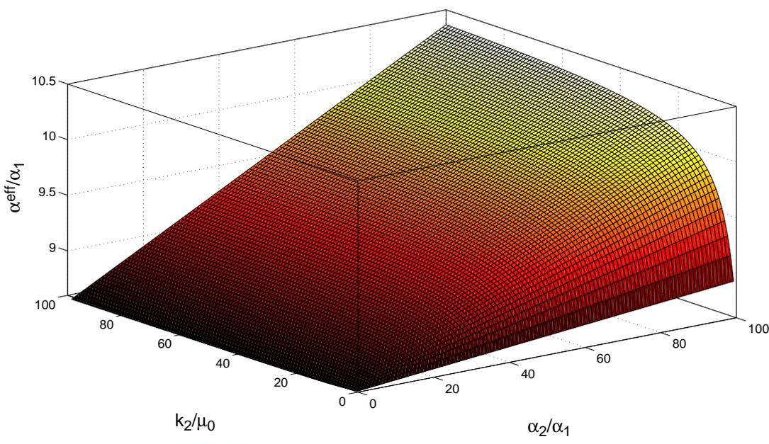
Figure 9. Normalized effective thermal expansion coefficient  $\alpha_{eff}/\alpha_1$  of a composite material made of coated inclusions as described in Fig. 4: result from the present model using Levin's formula (eq.(58)) with  $f_1 = 0.1$ ,  $f_2 = 0.01$ . The elastic properties of the different phases are characterized by:  $k_1/\mu_0 = 15$ ,  $\mu_1/\mu_0 = 7$ ,  $k_0/\mu_0 = 2$ ,  $\mu_2/\mu_0 = 4$  and  $\alpha_0/\alpha_1 = 10$ .
