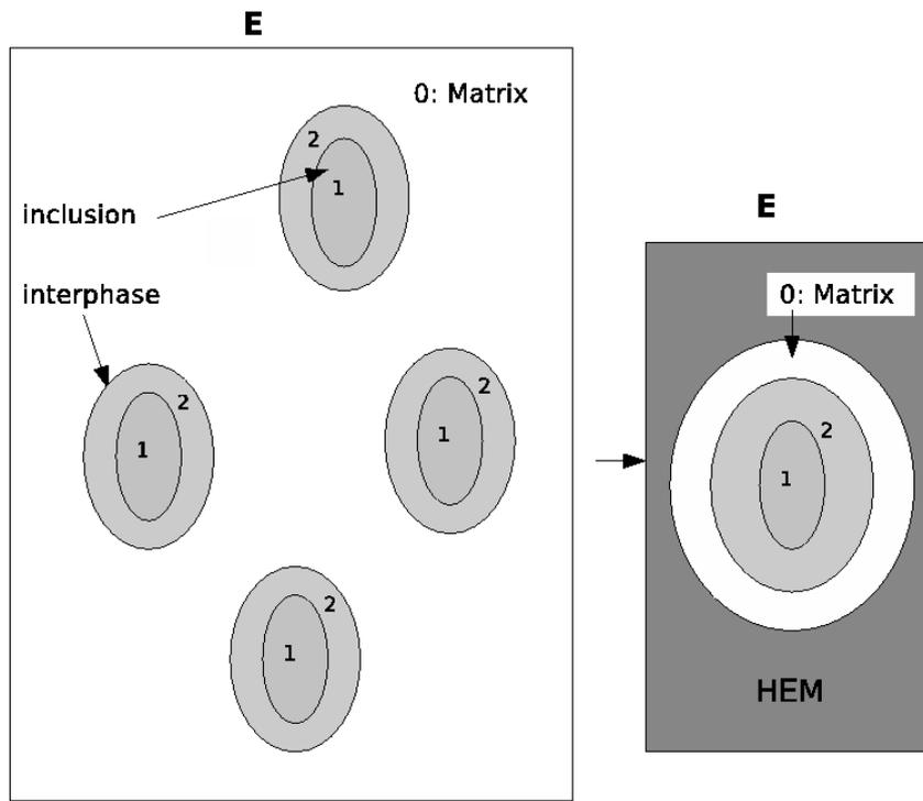
28 Figure 4. Schematic principle of the "4-phase" scheme (self-consistent condition). The inclusion phase
