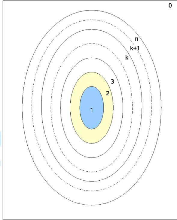
Figure 1. Multi-coated inclusion problem with eigenstrains considering  $n$  phases. The inclusion is embedded in an infinite reference medium (0). In this description, Phase 2 is called the *interphase* when  $n = 3$  for instance.
