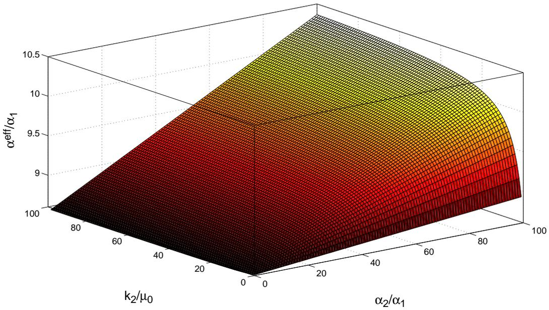
Figure 7. Normalized effective thermal expansion coefficient  $\alpha_{eff}/\alpha_1$  of a composite material made of coated inclusions as described in Fig. 4: result from the present model (eq.(57)) with  $f_1 = 0.1$ ,  $f_2 = 0.01$ . The elastic properties of the different phases are characterized by:  $k_1/\mu_0 = 15$ ,  $\mu_1/\mu_0 = 7$ ,  $k_0/\mu_0 = 2$ ,  $\mu_2/\mu_0 = 4$  and  $\alpha_0/\alpha_1 = 10$ .
