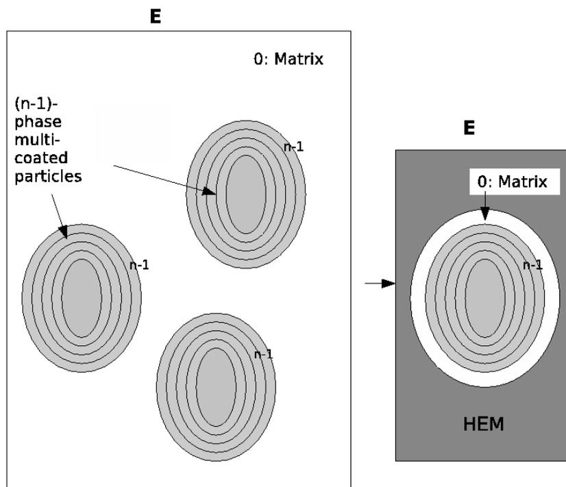
Figure 3. Schematic principle of the "(n + 1)-phase" model (self-consistent condition).
