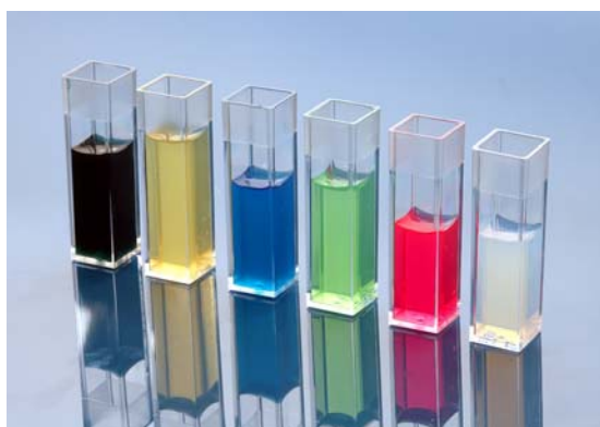
Fig 6 : Lipidots® lipid nanoparticles containing various organic dyes for molecular imaging. Credit: CEA-Leti
