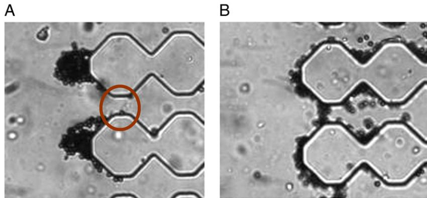
**Fig. 11.** Observation of the first stages of the particle capture. (A) After a PDMS conditioning with a KCl solution (image taken 1 min after the beginning of the filtration experiment). (B) After a PDMS conditioning with ultrapure water (image taken 30 s after the beginning of the filtration experiment). The formation of arches at the entrance of microchannels is clearly seen in image (B), whereas such a capture is not seen in (A).
