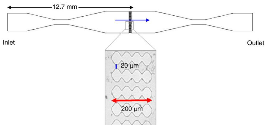
**Fig. 6.** Sketch of the PDMS micro-separators (top) with an image centered on some of the microchannels (bottom). The whole filtering part of the device consisted of a parallel arrangement of 27 microchannels.
