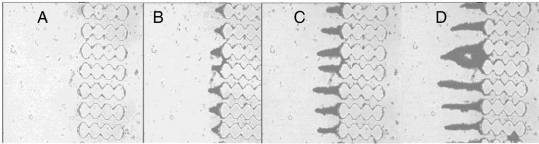
**Fig. 9.** Observation of particle capture after a conditioning of the micro-separator with a KCl solution, leading to the formation of dendrites. Image A was taken at  $t_0 + 1$  min (at  $t_0$ , the suspension starts flowing into the microchannels), image B at  $t_0 + 20$  min, image C at  $t_0 + 45$  min and image D at  $t_0 + 90$  min.
