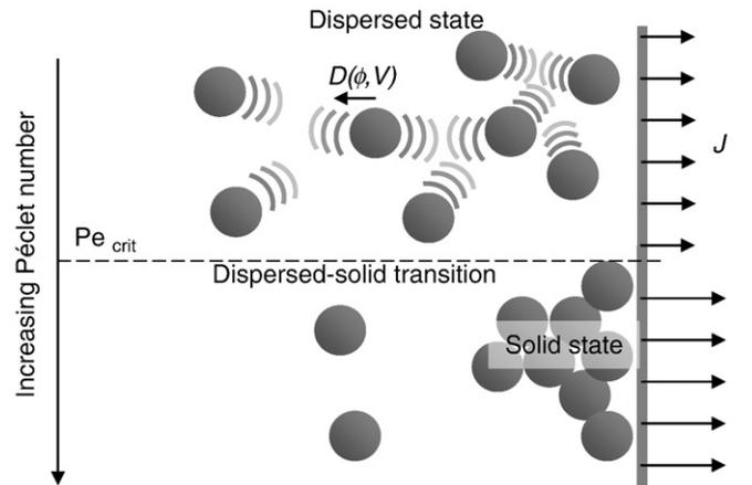
Fig. 3. Schematic representation of the links between colloidal surface interaction, phase transition, osmotic pressure and critical operating conditions for concentration processes.
