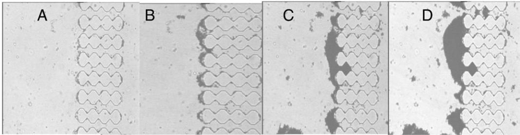
**Fig. 10.** Observation of particle capture after a conditioning of the micro-separator with ultrapure water, leading to the progressive obstruction of the microchannels, and then formation of a filtration cake. Image A at  $t_0 + 1$  min, image B at  $t_0 + 20$  min, image C at  $t_0 + 45$  min and image D at  $t_0 + 90$  min.
