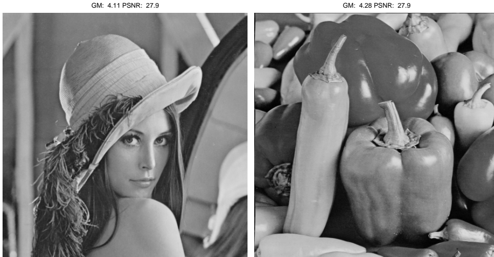
Figure 16: “Lena” and “peppers” after the same geometrical distortion. The left image is visibly corrupted (look at the vertical structure on the left), while the right one looks perfect. The PSNR is not able to catch the perceptual quality difference of these images, while the GM is, as shown in Table 2
