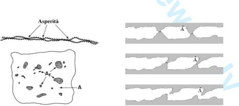
Fig. 3. Topography of surfaces and deformation of asperities in the adhesive junctions model
