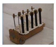
**Fig. 4.** Cart equipped with a variety of metal blades. When the cart collides against a wall, most of the translational kinetic energy of the cart is transferred to the blades, which start oscillating, so that the collision becomes strongly inelastic and the rebound speed is almost zero.
