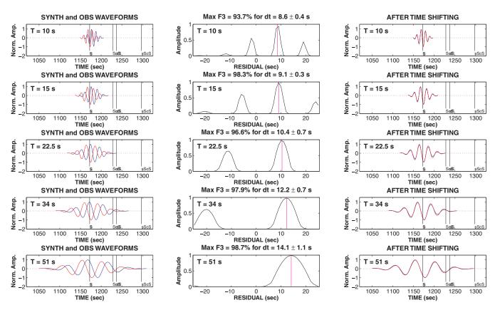
**Figure 1.** Measuring multiple-frequency time residuals. Left column: observed (blue) and synthetic (red) isolated and tapered *S*-phase waveforms (corresponding to Fig. A1a). Middle column: for each filtering period (T),  $F_3(\tau)$  is maximized for a delay-time  $\tau_m(T)$ . Right column: observed and synthetic waveforms after time shifting of  $\tau_m(T)$ . Note that each raw corresponds to a different filtering period T.
