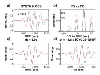
**Figure B1.**  $F_3(\tau)$  versus  $\gamma_{d,s}(\tau)$  for a *S*-wave recorded at station ATD (Geoscope network), event 2004 October 15. (a) Observed and synthetic waveforms filtered at 10 s period. (b)  $F_3(\tau)$ , in black, versus  $\gamma_{d,s}(\tau)$ , in magenta. Note that  $F_3(\tau)$  has secondary maximums lower than for  $\gamma_{d,s}(\tau)$ . (c) Waveforms after appropriate time-shifting. (d) Waveforms after wrong time-shifting, corresponding to a cycle-skip.
