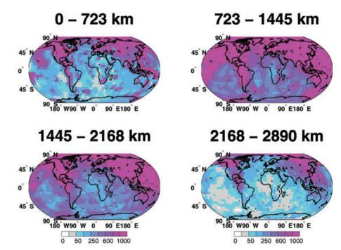
Figure 3. Ray density maps per  $6^{\circ} \times 6^{\circ}$  cells, shown at four different depth slices. The colourscale represents the number of rays in each cell, normalized by the cell size. Cells with less than 10 rays are shown in white.
