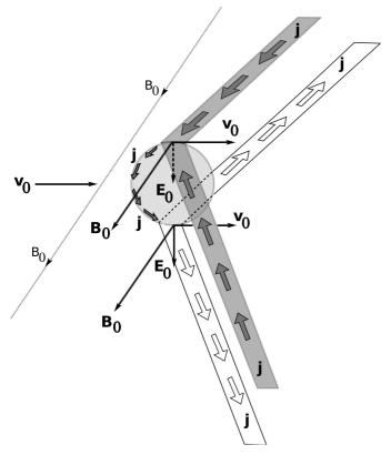
Fig. 1. Schematic view of an unipolar inductor.
