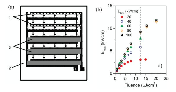
Figure 2 (a) Schematics of the THz emitting MSM. 1: interdigitated finger electrodes, 2: SI GaAs substrate, 3: opaque metallization shadowing one electric field direction. The electric field direction is indicated by arrows [45]. (b) peak THz electric field as a function of excitation fluence on the photoconductor for different acceleration fields at 250 kHz repetition rate [46].
