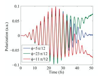
Figure 4:Time dependent polarization for Ar atoms subjected to 800 nm + 400 nm optical pulses with various values of the relative phase  $\phi$  between the two components. Asymmetric polarization occurs for values of  $\phi$  close to integer multiples of  $\pi$ . After Ref. [50], used with author's permission.
