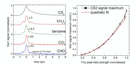
Figure 11: (a) Terahertz-induced birefringence in polarizable liquids. In the time domain, the signal follows the square of the THz pulse. (b) The peak signal scales quadratically with the THz field strength, demonstrating the  $\chi^{(3)}$  nature. From [24]
