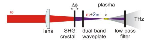
Figure 3. Scheme of the experimental realization of the two-color THz generation in plasma gas targets.  $\Delta \phi$  indicates the relative phase between the fundamental and its second harmonic, which can be varied e.g. by translating the SHG crystal.
