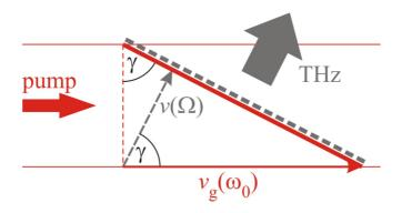
Figure 6 Velocity matching using TPFP. The thick red/solid line indicates the pump pulse front, the thick grey/dashed line indicates the THz phase front. The arrows indicate the propagations direction and velocities of these two surfaces.
