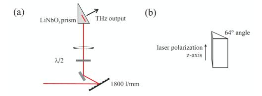
Figure 8 (a) Experimental setup for THz generation by TPFP in LN. (b) LN crystal orientation.
