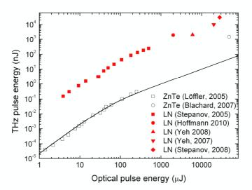
Figure 9: Scaling of the output THz pulse energy with the pump pulse energy for sources based on LN (with TPFP), and ZnTe. The solid line is a fit using model described in the text. Löffler 2005 [94], Blanchard 2007 [76], Stepanov 2005 [95], Hoffmann 2010 [97], Yeh 2008 [91], Yeh 2007 [90], Stepanov 2008 [96].
