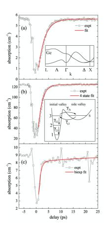
Figure 10: Dynamic behavior of the saturation of free-carrier absorption in the n-type semiconductors Ge, GaAs and Si. Plotted is a frequency averaged (0.2-2.0 THz) absorption coefficient. The solid lines are fits using a simple rate equation model [22].
