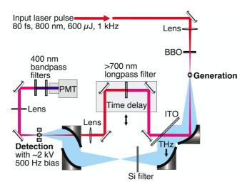
Figure 5. Schematic diagram of the experimental setup for coherent THz generation and detection in plasmas (from [63], used with permission)
