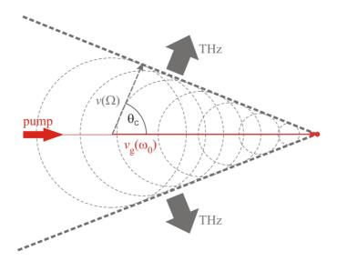
Figure 7 Cherenkov-like cone of emitted radiation due to OR of a subpicosecond optical pulse moving at a velocity  $v_g(\alpha_0)$ , which is greater than the THz phase velocity  $v(\Omega)$ , of the emitted radiation. After Ref. [86].
