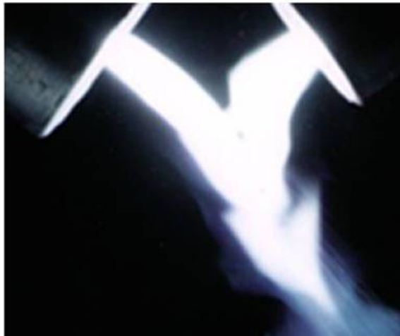
Figure 8 Diagram showing the image of a typical twin-torch plasma. The thinner jet originates from the cathode and the bent jet is from the anode.
