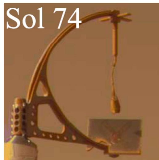
Figure 12. Image of the telltale used to determine estimates of winds at the Phoenix landing site. Adapted from Holstein-Rathlou et al. [2010] with permission.
