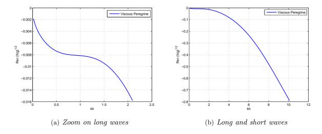
Figure 3. Real part of the wave frequency  $\tau$  with zoom on long waves region on the left image. The real part of the phase velocity of full Euler equations is identically equal to zero since the fluid is assumed to be perfect.
