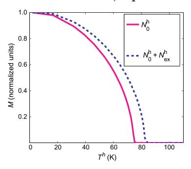
**Figure 1.** Temperature dependence of the normalized equilibrium ion magnetization for two hole densities. Here  $N_{\rm ex}^{\rm h} = 5 \times 10^{19} \, {\rm cm}^{-3}$ .
