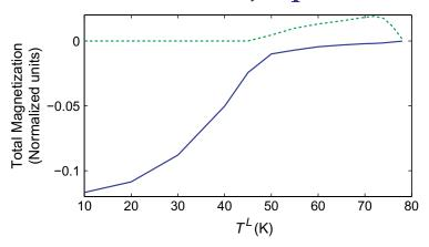
**Figure 4.** Minimum (solid line) and maximum (dashed line) of the total magnetization for different lattice temperatures.
