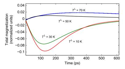
**Figure 3.** Time evolution of the total magnetization for different lattice temperatures:  $T^{L} = 10 \,\mathrm{K}$  (red line),  $T^{L} = 30 \,\mathrm{K}$  (green line),  $T^{L} = 50 \,\mathrm{K}$  (black line) and  $T^{L} = 70 \,\mathrm{K}$  (blue line).
