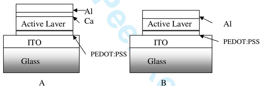
Fig.5. Schemes of single-layer EL (A) and PV(B) devices.
