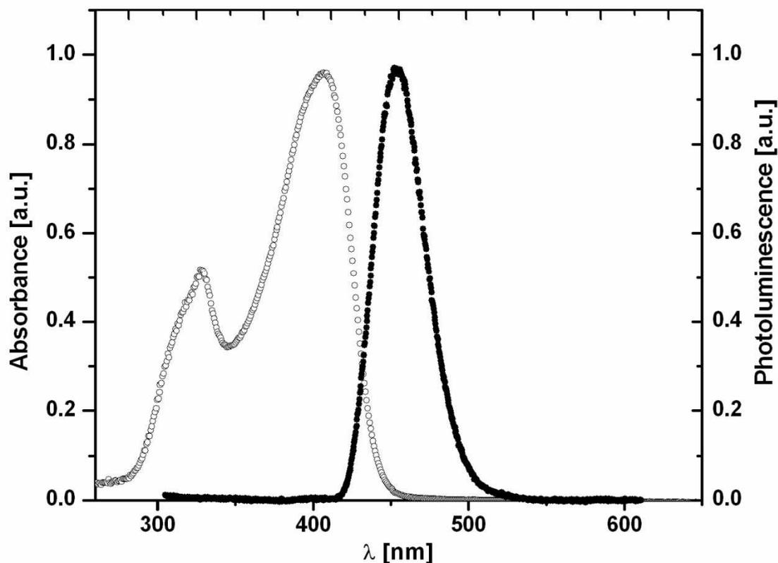
Fig.4. Measured absorption (open circles) and photoluminescent spectra (solid circles) of SM dissolved in THF solution
