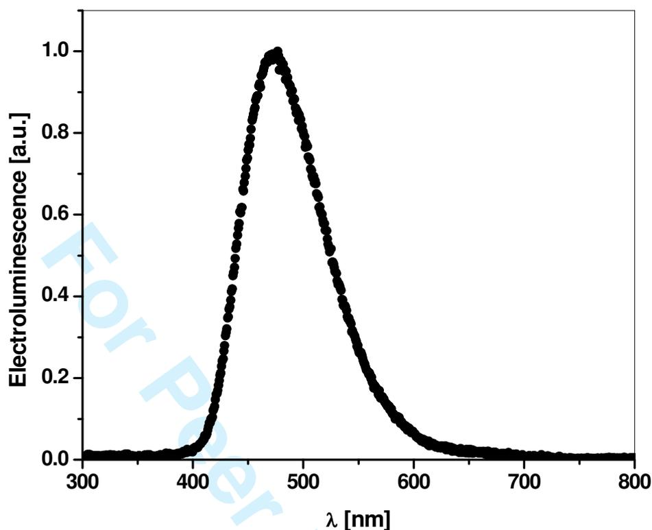
Fig.6. Electroluminescent spectrum of the device based on star-burst PQ
