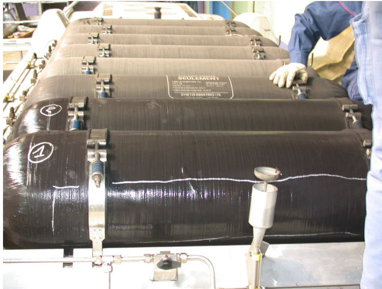
Figure 1: Natural gas cylinders made from carbon fibre reinforced epoxy resin on the roof of a bus.
