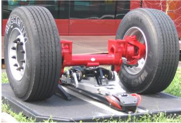
Fig. 2 Central guidance system mounted on the wheel axle
