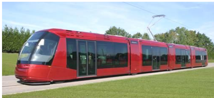
Fig. 1 The tramway on tires (STE4) used in the city of Clermont-Ferrand - France
