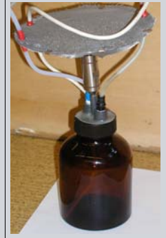
Sampling bottle, valve and "area lysimeter"
