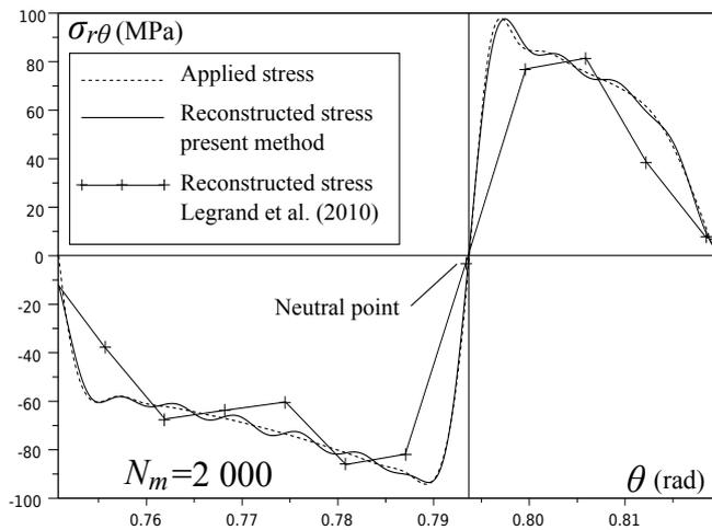
Figure 19: Results for cold rolling without noise,  $\sigma_{r\theta}$
