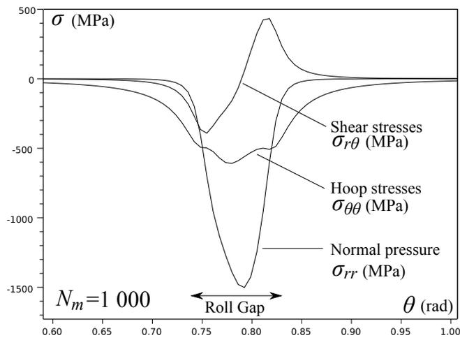
Figure 13: Stresses calculated at  $R_c$  for cold rolling
