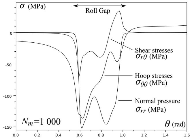
Figure 12: Stresses calculated at  $R_c$  for hot rolling
