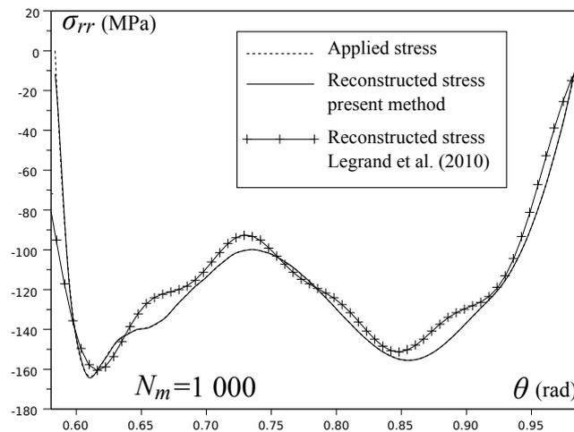
Figure 15: Results for hot rolling without noise,  $\sigma_{rr}$
