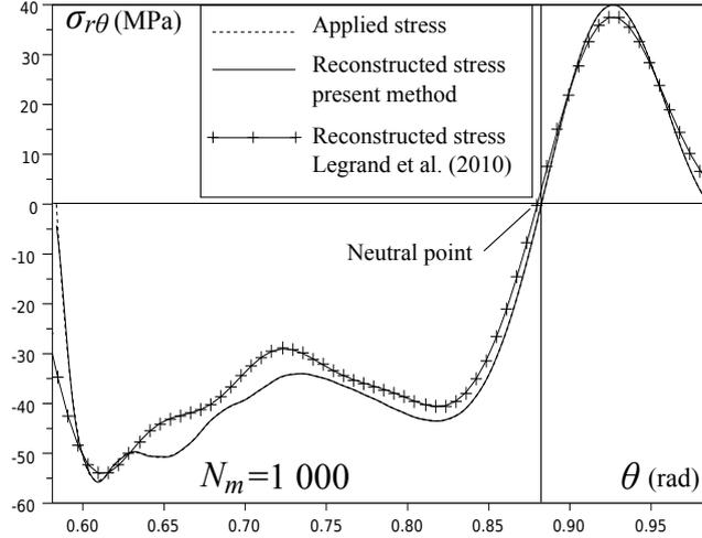
Figure 16: Results for hot rolling without noise,  $\sigma_{r\theta}$
