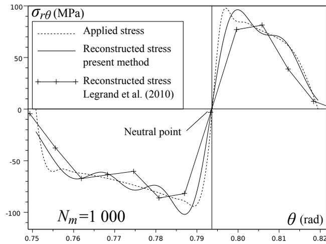
Figure 18: Results for cold rolling without noise,  $\sigma_{r\theta}$
