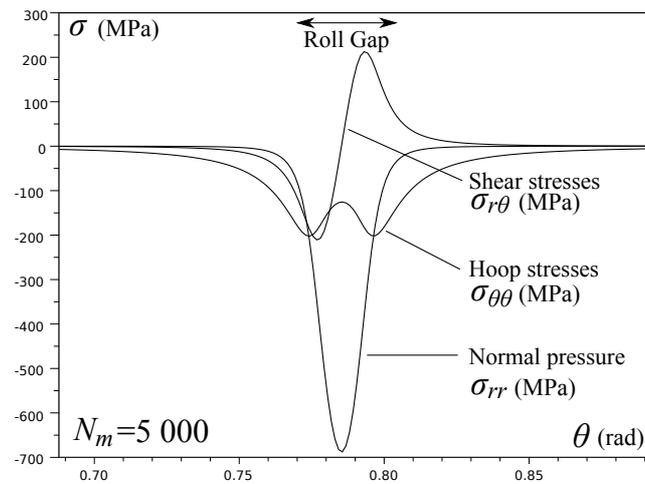
Figure 14: Stresses calculated at  $R_c$  for temper-rolling
