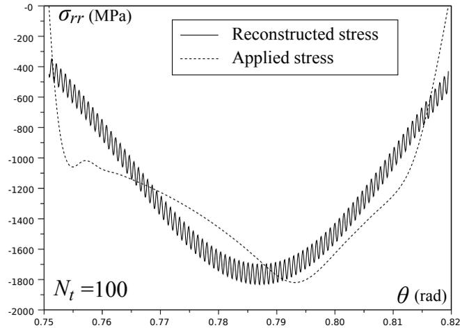
Figure 3: Reconstruction for cold rolling conditions with  $N_m = 1000$  and  $N_t = 100$
