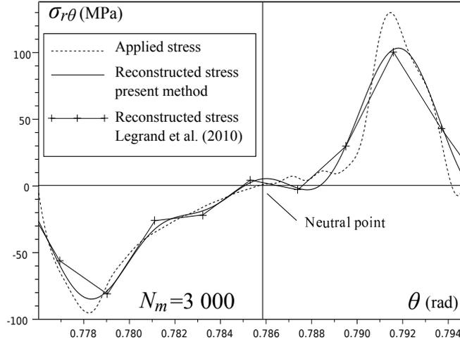
Figure 21: Results for temper-rolling without noise,  $\sigma_{r\theta}$
