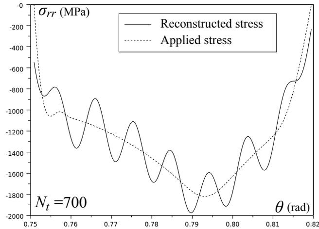
Figure 5: Reconstruction for cold rolling conditions with  $N_m = 1000$  and  $N_t = 700$
