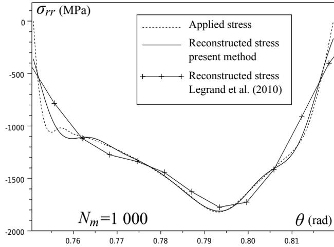
Figure 17: Results for cold rolling without noise,  $\sigma_{rr}$
