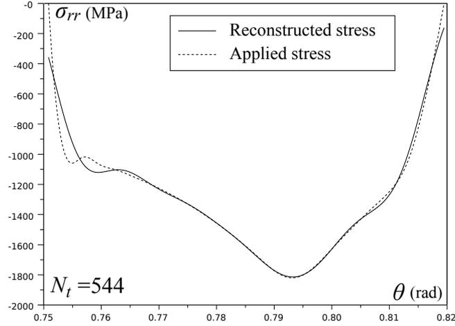
Figure 4: Reconstruction for cold rolling conditions with  $N_m = 1000$  and  $N_t = 544$
