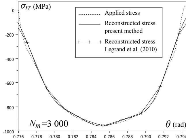
Figure 20: Results for temper-rolling without noise,  $\sigma_{rr}$
