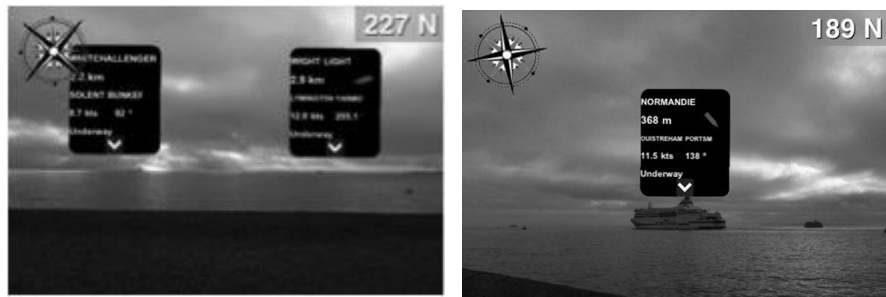
(a) Scene augmented with AIS information. (b) A vessel augmented with AIS information
