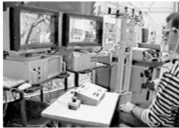
Fig. 1.5: The teleoperated robot is displayed simultaneously in real 3D images and using 3D artificial images.
