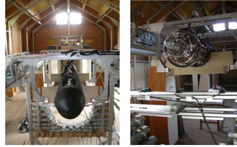
Fig. 4. Submarine Mock-up placed on the railway in the LMMCF. On the left, the mock-up in the simulator. On the right, only internal hull is shown with degaussing coils and fixed external fluxgate sensors.
