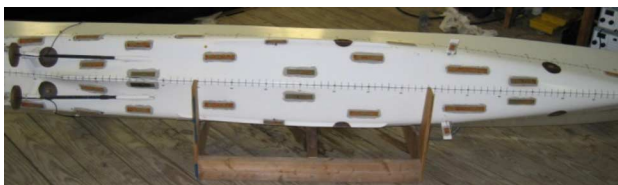
Fig. 7. 1:40th ship mock-up (underside) with rectangular cathodes and anodes in round dielectric patches.
