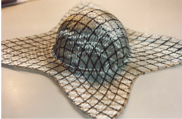
Figure 1. Hemispherical preforming of a woven composite reinforcement. A network of initially straight and continuous orthogonal lines has been drawn on the initial flat reinforcement.
