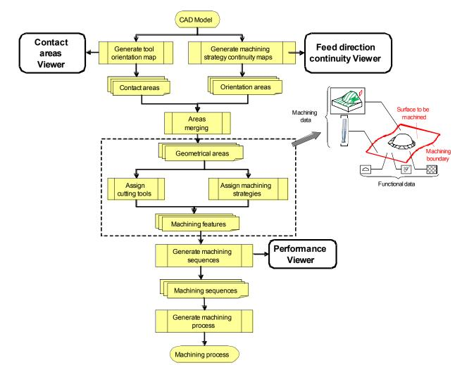
Fig. 15. Machining process generation with knowledge integration
