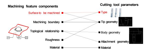
Fig. 10. Machining features and cutting tool links
