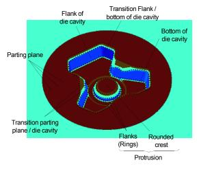
Fig. 22. Geometric features extraction
