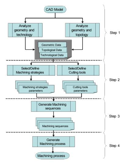
Fig. 3. Machining process generation
