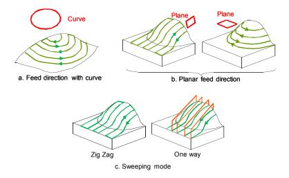
Fig. 6. Machining types and parameters
