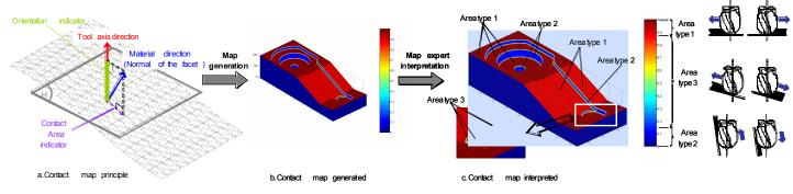
Fig. 17. Elementary geometrical feature identification
