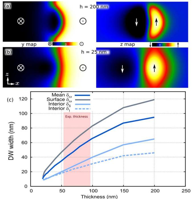
Figure 4. Domain wall width measure with respect to the thickness on simulated iron bar. (a)  $y$ - and  $z$ -components of the magnetization on a wall profile for a 200 nm-thick iron bar. (b) Same as in (a) for a 25 nm-thick iron bar with same aspect ratio. (c) Plot of the wall width versus thickness using various description of the domain wall width (see text). Experimental thicknesses area is reported on the graph.
