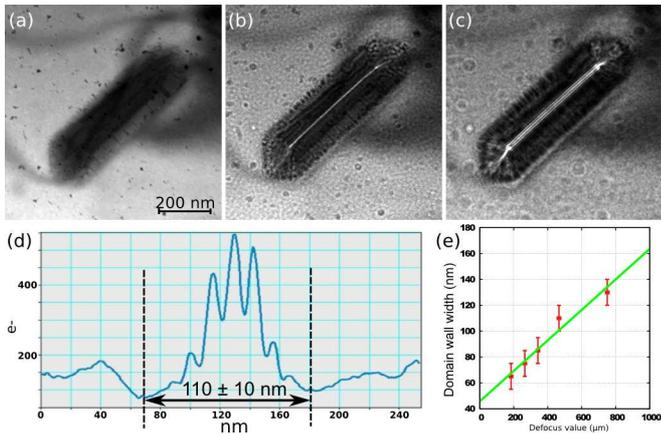
Figure 3. (a-c) Images of a Fe (110) dot for different defocus values (from (a) to (c) values of defocus are 0, 10 and 30  $\mu\text{m}$  respectively). The thickness of the dot was estimated (see in the text) to 90 nm. (d) Intensity profile of the convergent wall obtained from (c) and associated width measurement (see text). (e) Zero-defocus approximation for domain wall width measurement.
