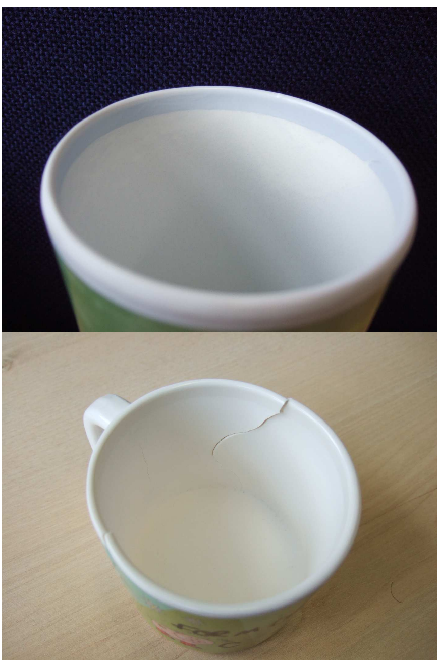
Figure 1 Examples of discoloured/pitted/cracked melaware
