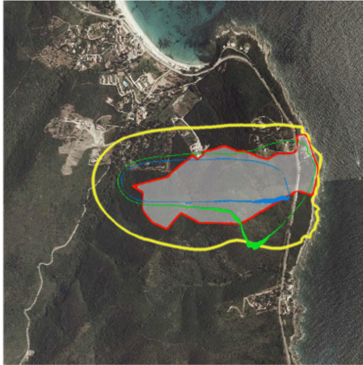
Fig. 14. CASE A: Simulations results and observations for the Favone fire. Blue: simulated fire contour at 15:50 (after 50''), Green: simulated contour at 19:00, yellow: simulated contour at 19:00 (non coupled) ; Red: final observed contour of the fire.
