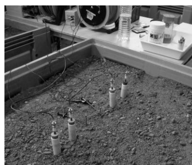
Figure 4: Electrode positions at the soil surface in a container.
