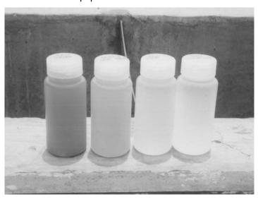
Figure 1: Improved water quality along MSF system (samples from: raw water, settling tank, pre-filter, slow sand filter – left to right).
