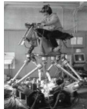
Fig. 5. Parallel platform based motorcycle simulator developed in Japan
