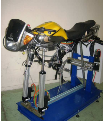
Fig. 9. The developed riding motorcycle simulator by INRETS-UEVE
