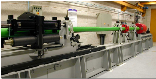
Fig. 1: Gas launcher and deformable projectile (about 5 kg)
