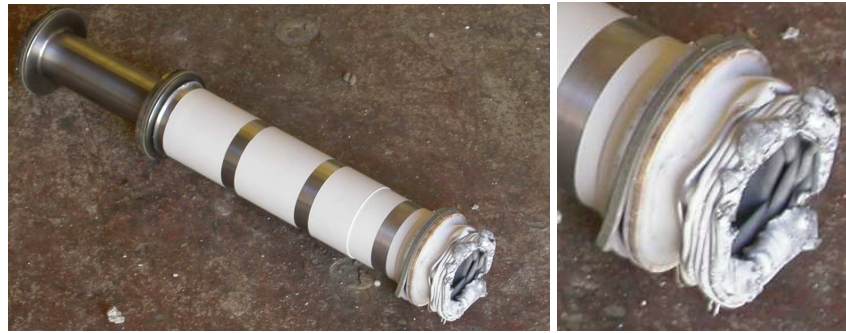
Fig. 4: Deformation of the missile after perforation (test n°2, V_0 = 70.2 m/s)
