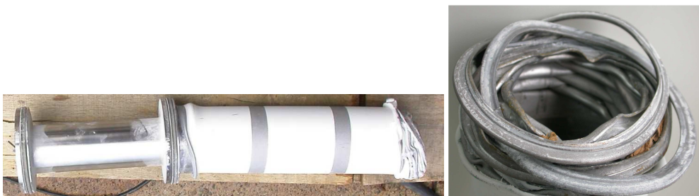
Fig. 2: Deformation of the missile after perforation (test n°1, V_0 = 107.5 m/s)
