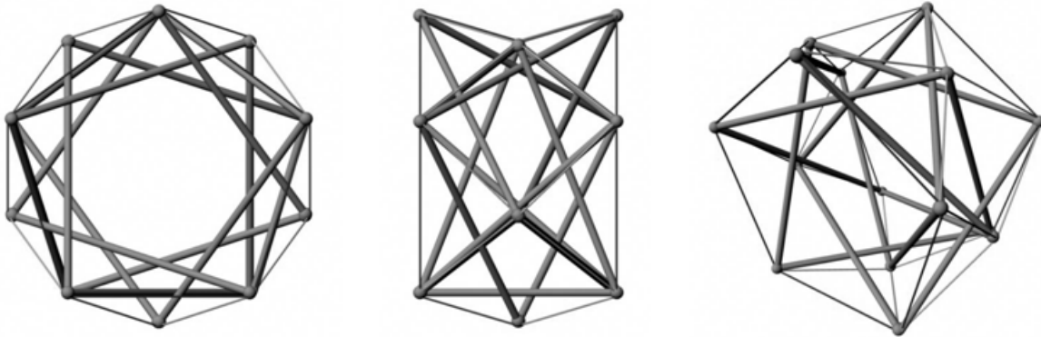
FIG. 1 – Illustration of a pentagonal tensegrity-ring module including struts, layer cables and x-cables
