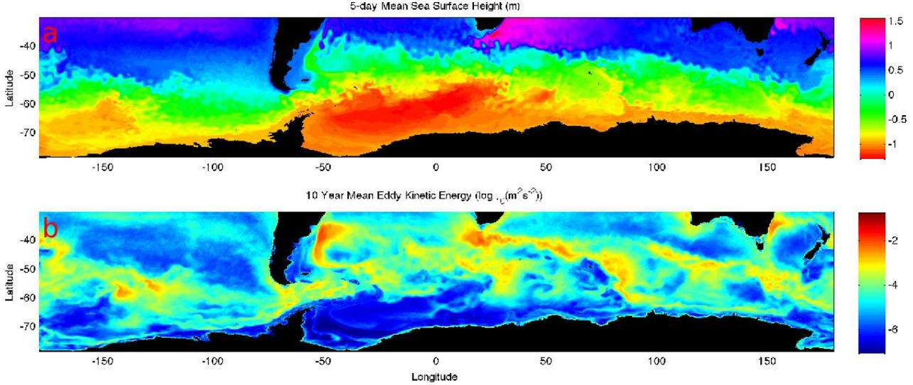
**Figure 1.** Surface properties of PERIANT8: a) Sea surface height for the final 5-days of simulation (27th – 31st of December 2007). b)  $\text{Log}_{10}$  of mean eddy kinetic energy for the final 10 years (1998–2007)
