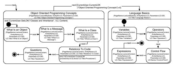
Figure 3.5 Excerpt of UML-Guide state diagram extended with tagged values representing WebML concepts.
