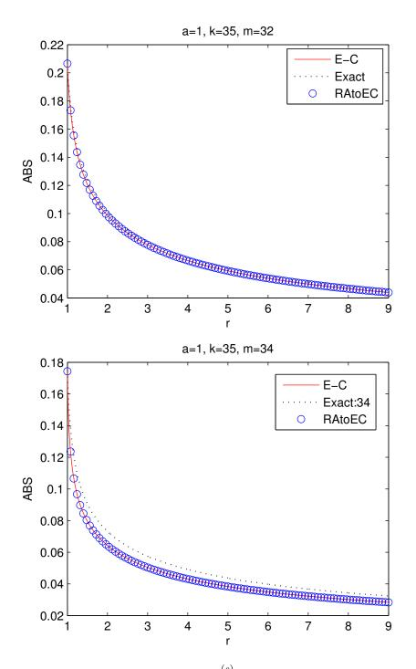
Figure 10: Magnitude of the scattered waves  $u_m^{(s)}$  (along a certain direction) for a circular cylinder with m = 32 and 34.
