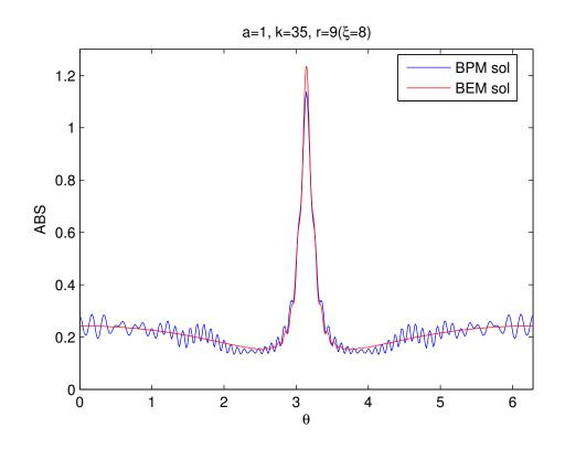
Figure 4: Magnitude of the scattered wave of a circular cylinder at r = 9.
