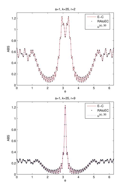
Figure 8: Magnitude of the scattered wave of a circular cylinder for the incident field truncated to 30 terms.
