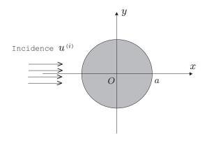
Figure 3: The scattering problem of a circular cylinder.
