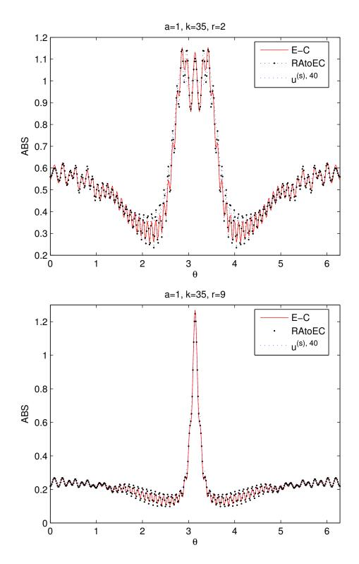
Figure 9: Magnitude of the scattered wave of a circular cylinder for the incident field truncated to 40 terms.
