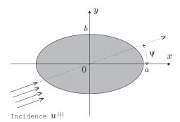
Figure 5: The scattering problem of an elliptic cylinder for plane incident wave with an incident angle  $\psi$ .
