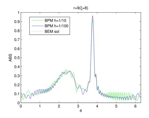
Figure 6: Magnitude of the scattered wave of an elliptic cylinder for a plane incident wave with  $\psi = 35^o$ .
