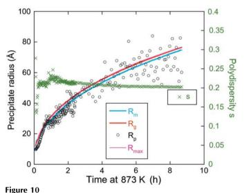
Parameters extracted from the scattering curves through the whole 873 K heat treatment on the Fe–Cu alloy.
