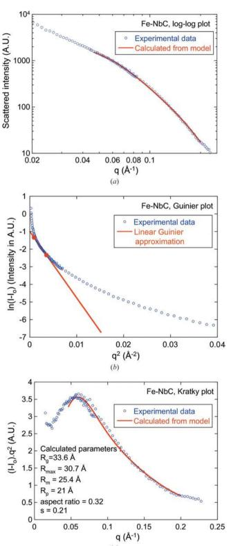
**Figure 11** Magnetic scattering data for the Fe–Nb–C alloy. (a) Raw scattering curve, along with a fit for a model containing plate-like ellipsoidal precipitates. (b) Guinier plot. (c) Kratky plot and the calculated parameters of the microstructure.
