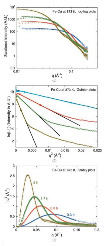
Figure 9 Scattering curves for four selected ageing times (0.3, 0.8, 1.7 and 3 h) during heat treatment at 873 K on the Fe–Cu alloy. (a) Raw scattering curves (symbols) and model fitting curves (solid lines). (b) Guinier plot. The fitted straight lines were determined within the boundaries in a self-consistent way (see §2). (c) Kratky plot. The average radius  $R_{\rm m}$  and the polydispersity parameter were determined from the model fitting curves (solid lines).
