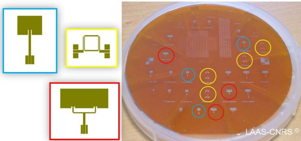
Fig. 6 Realized antennas and resonators on Kapton
