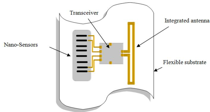
Fig. 1 Concept of the communicating nano-object on flexible film
