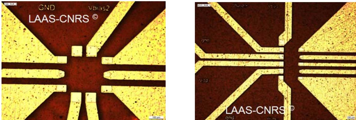
Fig. 5 Realized circuits on Kapton (location for the postponement of the dummy chip)
