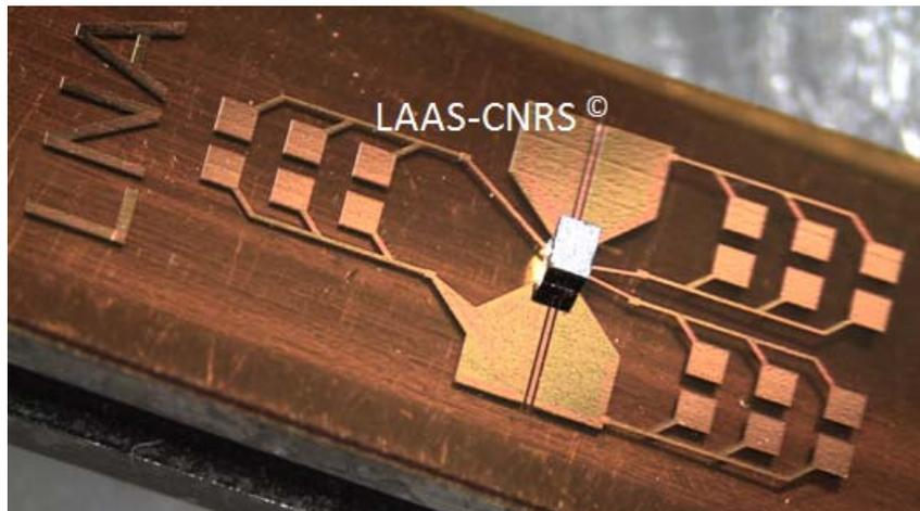
Fig. 8 First assembly tests (LNA Dummy on Kapton)
