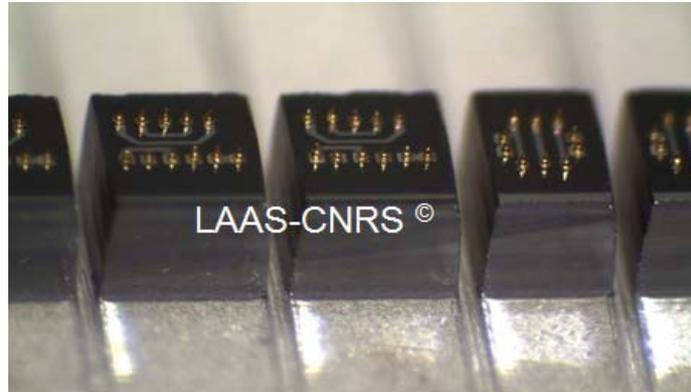
Fig. 7 Realized Silicon dummies (VCOs and LNAs)
