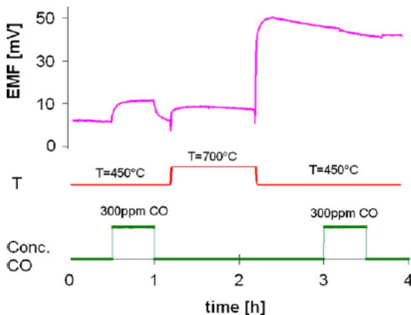
*Figure 7: Regeneration process of the catalytic layer (Pt1.7 = 1.7% Pt dispersed in alumina) in the presence of 12 vol.% O<sub>2</sub>, 2 vol.% H<sub>2</sub>O and N<sub>2</sub> balance.*
