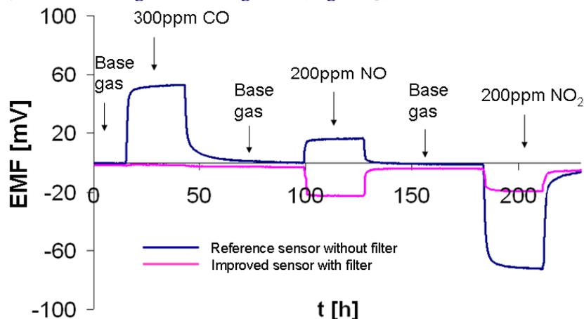
*Figure 5: Response of a sensor with a catalytic layer (Pt1.7 = 1.7% Pt dispersed in alumina) to CO, NO and NO<sub>2</sub> at 520 °C in the presence of 12 vol.% O<sub>2</sub>, 2 vol.% H<sub>2</sub>O and N<sub>2</sub> balance.*
