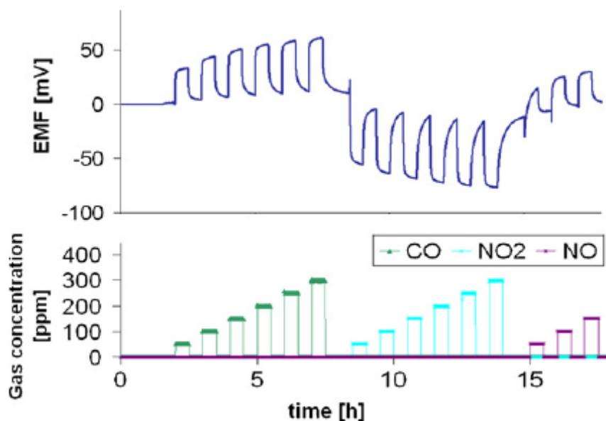
Figure 3: Sensor response to CO, NO and NO<sub>2</sub> at 450 °C (base gas: 12 vol.% O<sub>2</sub>, 2 vol.% H<sub>2</sub>O and N<sub>2</sub> balance).
