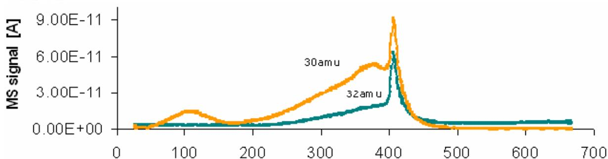
*Figure 8: TPD in helium of a 1.7% Pt dispersed in alumina catalyst after a pre-treatment of 12 h in 300 ppm NO<sub>2</sub>, 3.5% O<sub>2</sub> and He balance at 450 °C.*
