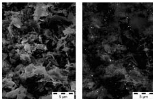
Figure 4: SEM of a deposited catalytic layer (Pt<sub>1.7</sub> = 1.7% Pt dispersed in alumina); left: secondary electron image; right: backscattering electron image.
