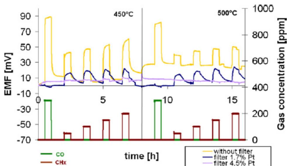
Figure 9: Sensor response to hydrocarbons (HC = 25% methane, 25% butane and 50% propene) at 450 °C and 500 °C, respectively, in the presence of 12 vol.% O<sub>2</sub>, 2 vol.% H<sub>2</sub>O and N<sub>2</sub> balance.
