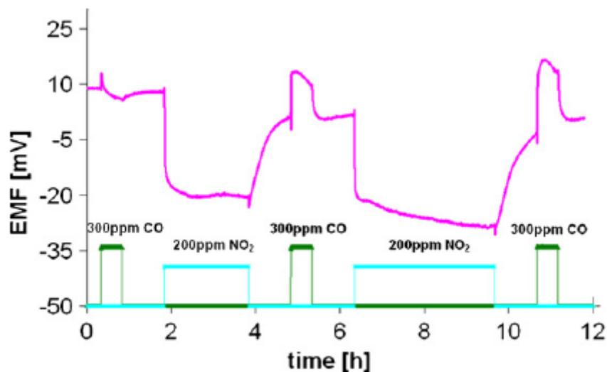
*Figure 6: Deactivation process of the catalytic layer (Pt1.7 = 1.7% Pt dispersed in alumina) at 450 °C in the presence of 12 vol.% O<sub>2</sub>, 2 vol.% H<sub>2</sub>O and N<sub>2</sub> balance.*
