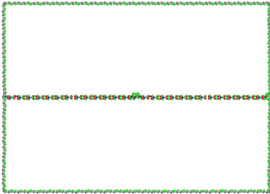
Figure 3. SCM of a \Sigma 17 symmetrical tilt boundary in copper at room temperature. Two periods of the simulated bicrystal are shown.
