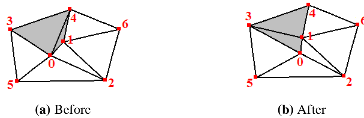
Fig. 4 Flip operation resulting from crossing the base line of the triangle during node 0 's movement towards node 2
