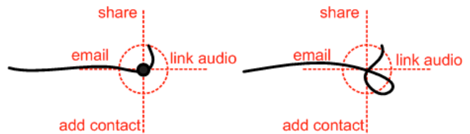
Figure 3. Left: Activating a selection with a marking knot Right: A pigtail [4]. Dotted lines show the frame of reference.
