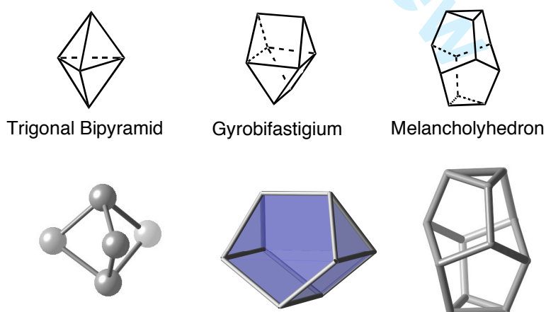
Figure 2. Structures of the carbon skeletons of bicyclopentane, cunneane and octahedrane, that approximate the geometry of the trigonal bipyramid, the gyrobifastigium, and the melancholyhedron, respectively.
