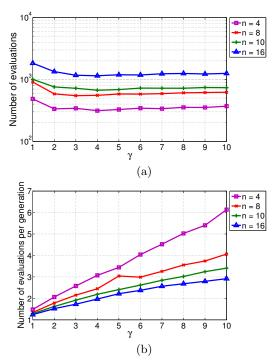
Figure 1: (a) Average number of evaluations of the p-sep lmm-CMA on  $f_{\text{Rosen}}^{100}$  to reach  $f_{\text{stop}}$  for varying population sizes  $\lambda = \gamma \times \lambda_{\text{default}}$ . (b) Average number of evaluations per generation of the p-sep lmm-CMA on  $f_{\text{Rosen}}^{100}$  for varying population sizes  $\lambda = \gamma \times \lambda_{\text{default}}$ .
