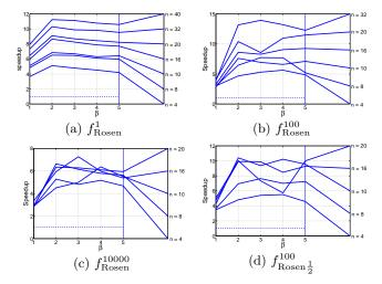
Figure 3: Average speedup with respect to CMA-ES to reach  $f_{\text{stop}}$  with a varying number of points used to build the meta-model  $k_i = \beta \times k_{i,\min}$  where  $k_{i,\min} = \frac{n_i(n_i+3)}{2} + 1$ . Each point corresponds to 20 runs performed.
