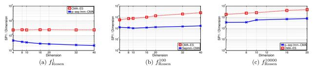
Figure 2: Success performance SP1 over the dimension of the problem on  $f_{\text{Rosen}}^{\alpha}$ , with  $\alpha = 1$ ,  $10^2$  and  $10^4$  for dimensions in between 4 and 40. The dimension of the sub-functions  $n_{\text{M}}$  equals 2.
