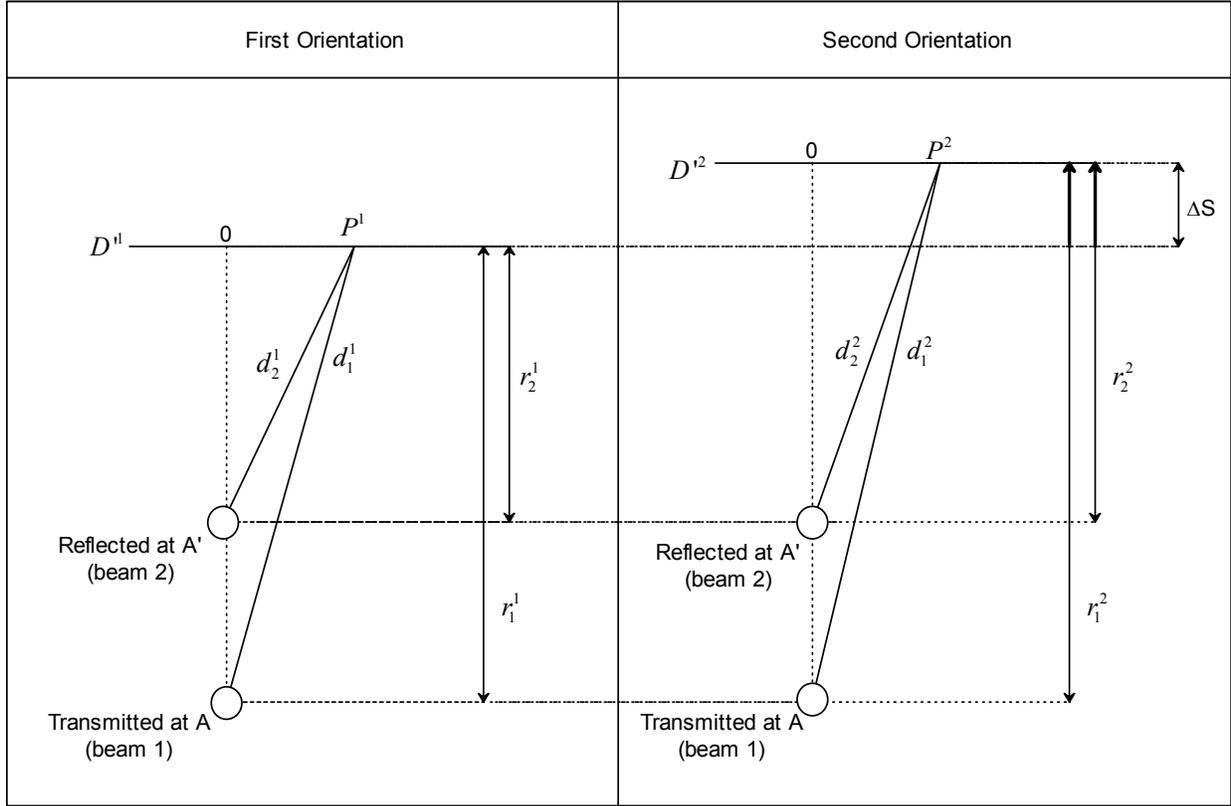
**Figure 3** In each orientation, the interference pattern is formed by two beams: one that is transmitted at A, and another that reflects at A', arriving both beams simultaneously at D'. The difference between the radii of the spheres is greater than zero and of constant value in both orientations. In the second orientation, both beams have to travel an additional distance  $\Delta S$  to arrive to D'.
