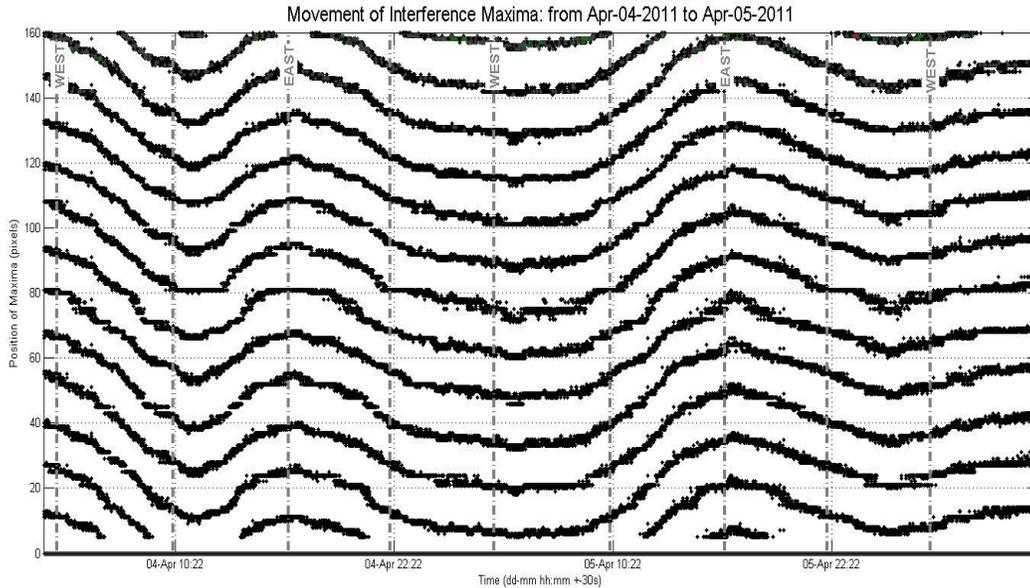
**Figure 6 Raw data plot of the experimental results done by the authors as verification to the presented formulation. The horizontal axis is time, the vertical axis is the vertical position on the screen of the interference pattern's maxima. Although the sinusoid are not perfect, it can be seen an apparent correlation between the sinusoid and the position of HIP24255 in the local "East" and "West".**
