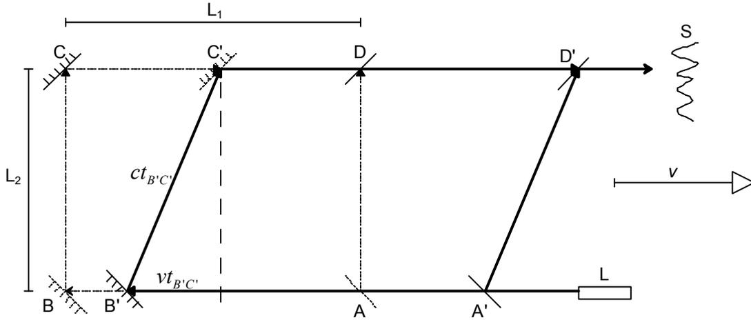
Figure 1 Interferometer by which calculations are made. Thin dotted lines represent the path light travels when the interferometer at rest ( $v=0$ ), thick solid lines represent the path light travels when the interferometer moves with  $v>0$ , the dashed line help visualize a right triangle of sides  $vt_{B'C'}$  and  $L_2$  and hypotenuse  $ct_{B'C'}$ .
