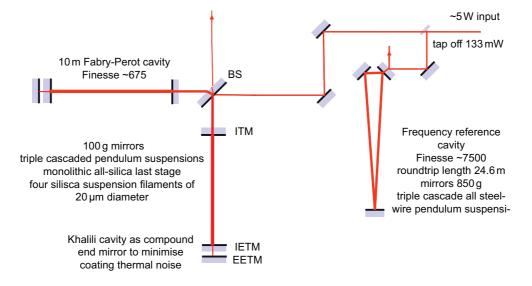
**Figure 2.** The basic optical layout for the first round of experiments in the AEI 10 m Prototype facility. Shown are the frequency reference cavity and the main interferometer along with the most relevant design parameters. Note, that only 5 W input power will be used for the first experiments.
