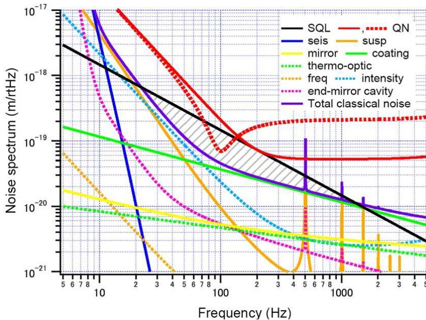
**Figure 3.** The design sensitivity of the AEI 10 m Prototype Interferometer. The black straight line is the SQL, the red solid curve is the sum of quantum noise, the blue solid line is the sum of all classical noise sources. The dashed area in between the sum of classical and quantum noise is the QND regime that we hope to be able to explore by applying e.g. the back-action evasion technique (red dashed curve).
