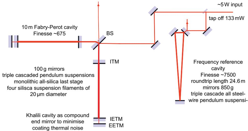
**Figure 2.** The basic optical layout for the first round of experiments in the AEI 10m Prototype facility. Shown are the frequency reference cavity and the main interferometer along with the most relevant design parameters. Note, that only 5 W input power will be used for the first experiments.
