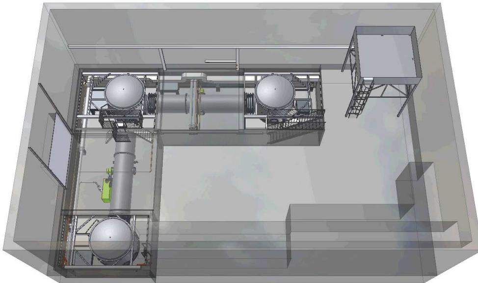
**Figure 1.** The vacuum system is set up in the downstairs area of the AEI prototype hall. The upstairs area is used for assembly of mechanical components before installation as well as for other optical experiments.
