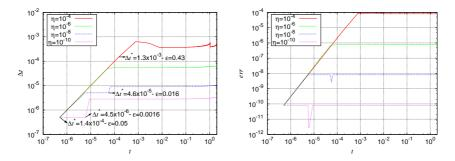
Fig. 6. BZ equation. Time evolution of accepted splitting time steps  $\Delta t$  (left) and local  $L^2$  error estimates  $err = \|S^{\Delta t}u_0 - S_{\varepsilon}^{\Delta t}u_0\|_{L^2}$  (right), for several tolerances  $\eta$ , considering critical  $\Delta t^{\star}$  and computation of  $\varepsilon$ .
