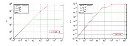
Fig. 5. BZ equation. Time evolution of accepted splitting time steps  $\Delta t$  (left) and local  $L^2$  error estimates  $err = \|S^{\Delta t}u_0 - S^{\Delta t}_{\varepsilon}u_0\|_{L^2}$  (right), for several tolerances  $\eta$  and  $\varepsilon = 0.05$ .
