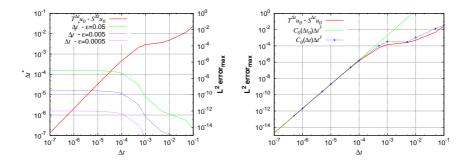
Fig. 4. BZ equation. Working region of the method  $\Delta t \leq \Delta t^*$  with  $\Delta t^*$  calculated with  $C_0$  estimated at  $\Delta t_0 = 10^{-5}$  and err obtained for several splitting time steps  $\Delta t$  and  $\varepsilon$  (left). Right: predicted Strang error calculated with  $C_0$  estimated at  $\Delta t_0 = 10^{-5}$  and locally at several splitting time steps  $\Delta t$ .
