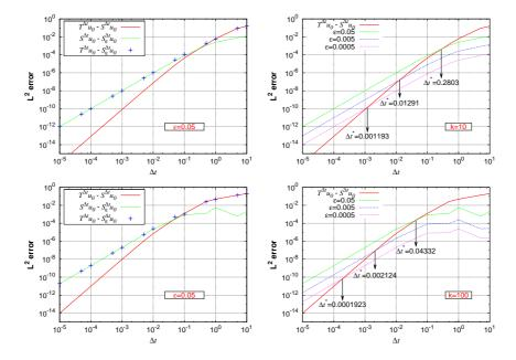
Fig. 2. KPP equation with k=10 (top) and k=100 (bottom). Local  $L^2$  errors for several splitting time steps  $\Delta t$  and  $\varepsilon=0.05$  (left). Right: critical splitting time steps  $\Delta t^\star$  obtained when  $\|T^{\Delta t}u_0-S^{\Delta t}u_0\|_{L^2} \approx \|S^{\Delta t}u_0-S^{\Delta t}_\varepsilon u_0\|_{L^2}$  in the numerical tests.
