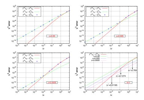
Fig. 1. KPP equation with k=1. Local  $L^2$  errors for several splitting time steps  $\Delta t$  and  $\varepsilon=0.05$  (top left), 0.005 (top right) and 0.0005 (bottom left). Bottom right: critical splitting time steps  $\Delta t^\star$  obtained when  $\|T^{\Delta t}u_0 - S^{\Delta t}u_0\|_{L^2} \approx \|S^{\Delta t}u_0 - S^{\Delta t}_{\varepsilon}u_0\|_{L^2}$  in the numerical tests.
