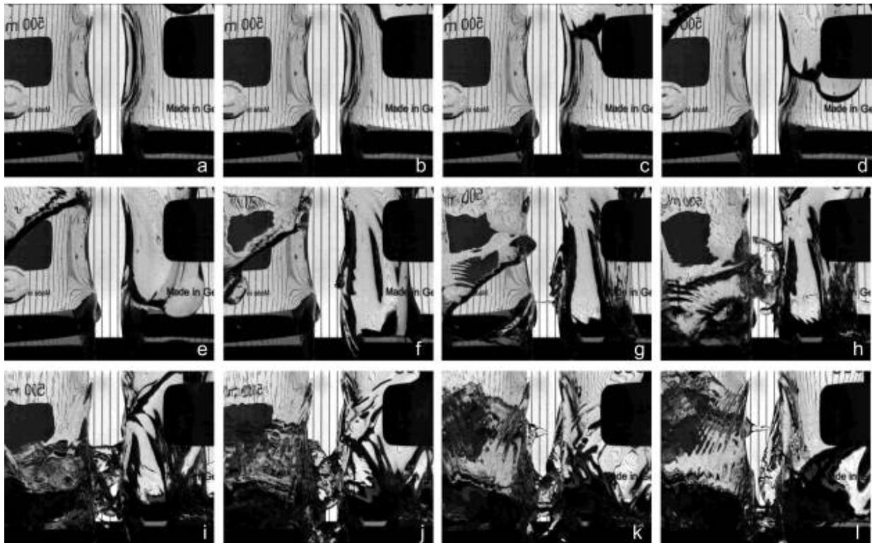
**Fig. 7:** Bridge formation under returning gravity. No bridge formation was observed in the absence of gravity (a), however the onset of gravitational acceleration (b-l) yielded multiple aqueous connections. The time between the images is 20 ms.
