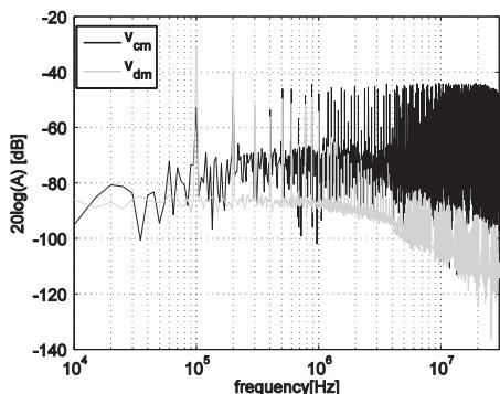
Fig.9. Impact of the isolation aging on DC-DC boost converter after 1k and more operation hours a) generated perturbation spectra
