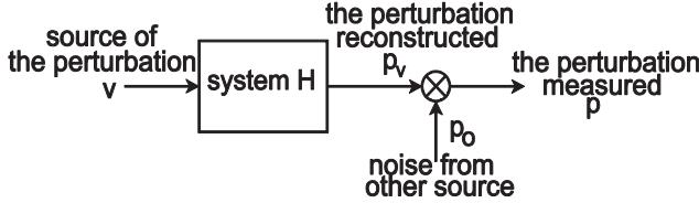
Fig.4. Wiener filtering in estimation of EMI
