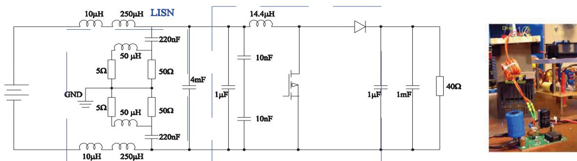
Fig. 1. Automotive DC-DC boost converter fed through the LISN: schematic diagram and experimental prototype view
