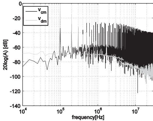
Fig.7. Impact of the input capacitor aging on DC-DC boost converter after 9k operation hours a) generated perturbation spectra
