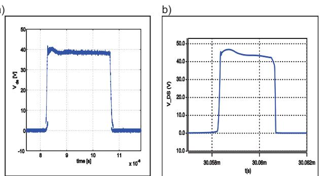
Fig.3. MOSFET voltage waveforms; a) measured b) simulated
