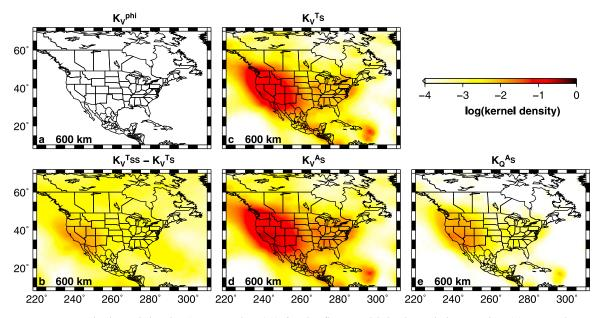
**Figure 6.** The kernel density (see equation (9)) for the five sensitivity kernels in equation (8) at 600 km depth. The heading indicates the kernel type. (a) For Love wave kernels and (b) for SS wave kernels. (c and d) For SH wave velocity kernels. (e) For SH wave attenuation kernels.
