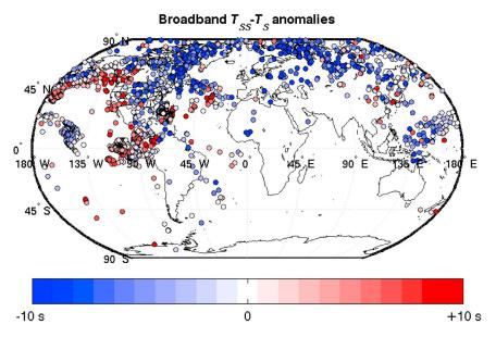
**Figure 2.** Broadband SS wave differential traveltime anomalies  $\delta(T_{SS} - T_S)$  plotted at each reflection point. Positive values reflect slow velocity anomalies in the vicinity of the reflection point, and negative values indicate fast velocity anomalies.
