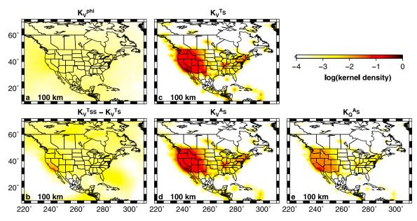
**Figure 5.** The kernel density (see equation (9)) for the five sensitivity kernels in equation (8) at 100 km depth. The heading indicates the kernel type. (a) For Love wave kernels and (b) for SS wave kernels. (c and d) For SH wave velocity kernels. (e) For SH wave attenuation kernels.
